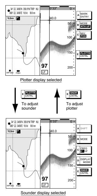
How to switch control between modes in the plotter/sounder combination display
